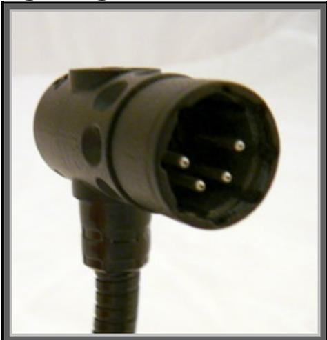
And of course, there is always someone ready to plug a microphone into any handy XLR connector, unless that connector is a "fool-proof" 4-pin variety existing for the sole purpose of accepting a Littlite XR-4 series gooseneck.
