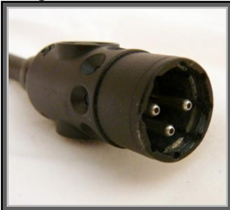
What looks like a low-impedance microphone input but isn't? It's a 12-volt task light connector on many large sound and lighting desks that's what! And it's a perfect place for an X series Littlite.
